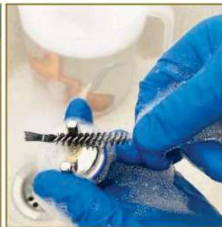
5 - Clean the air cap on each side with the brushes.
