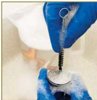
5 - Clean the air cap on each side with the brushes.
