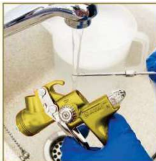
7 - Clean the needle with the brush.
