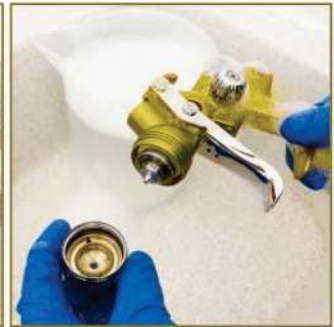
4 - Disassemble the needle and the air cap (see steps "Disassembly projector kit").
