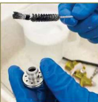
10 - Clean the nozzle on each side with the brushes.
