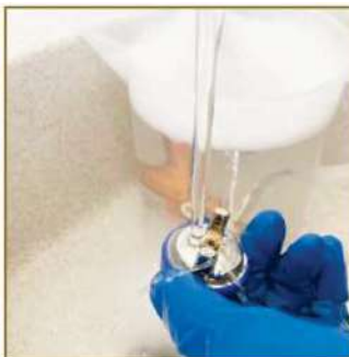
5 - Clean the air cap on each side with the brushes.
