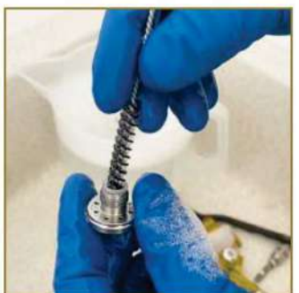
10 - Clean the nozzle on each side with the brushes.
