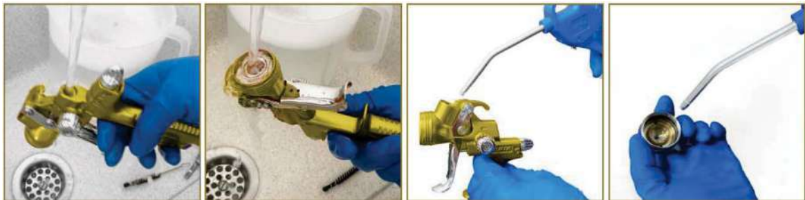
14 - Rinse the spray gun body and the product channel with clean water.
