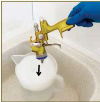
2 - Place the spray gun in the container
