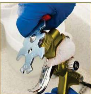
9 - Disassemble the nozzle (see steps "Disassembly of the projector kit").
