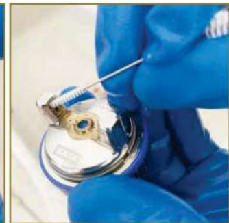
4 - Disassemble the needle and the air cap (see steps "Disassembly projector kit").
