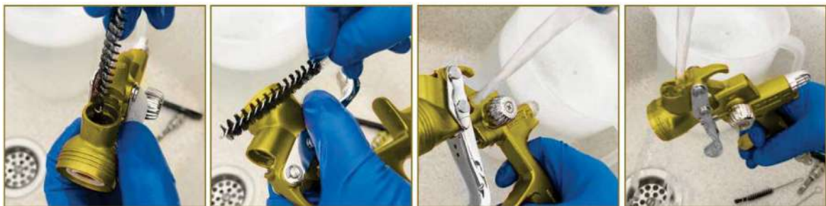
12 - Clean the spray gun body and product channel with the brushes
