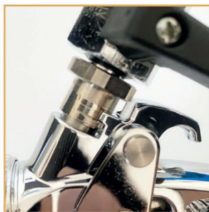
1 - Position the cup and insert it onto the spray gun
