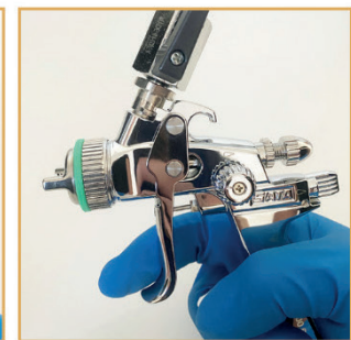
5 - Your cup is installed, open the cup valve by making a quarter turn, and you can spray your entremets.
