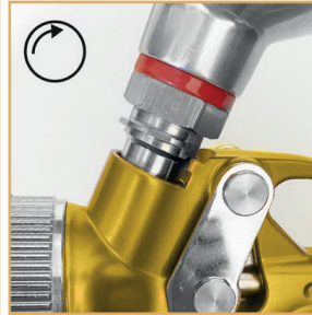
2 - Secure it by making a quarter turn, without forcing!
