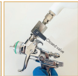
2 - Secure it by making a quarter turn, without forcing!
