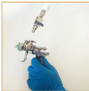
1 - Position the cup and insert it onto the spray gun
