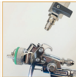
1 - Position the cup and insert it onto the spray gun
