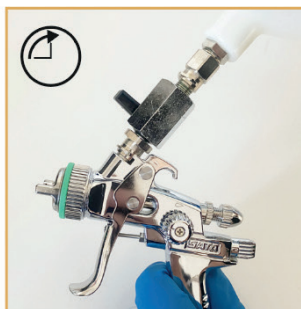
2 - Secure it by making a quarter turn, without forcing!
