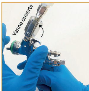
5 - Your cup is installed, open the cup valve by making a quarter turn, and you can spray your entremets.
