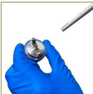
14 - Rinse the spray gun body and the paint channel with clean water. 15 - Dry using an air blower.
