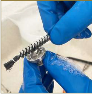
11 - Clean the nozzle on both sides using the cleaning brushes.
