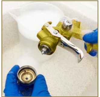
4 - Disassemble the needle and the air cap (see steps in "Nozzle Kit Disassembly").
