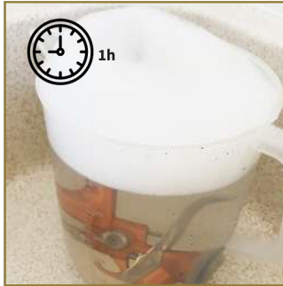
3 - Let the spray gun soak for 1 hour.
