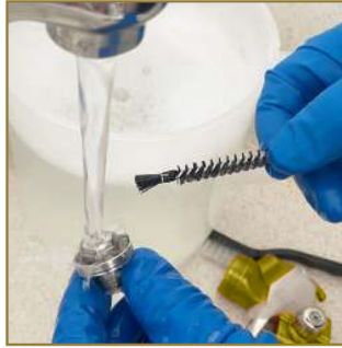
12 - Rinse the nozzle on both sides with clean water.
