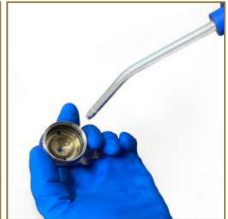
13 - Clean the spray gun body and the paint channel using the cleaning brushes. 14 - Rinse the spray gun body and the paint channel with clean water.
