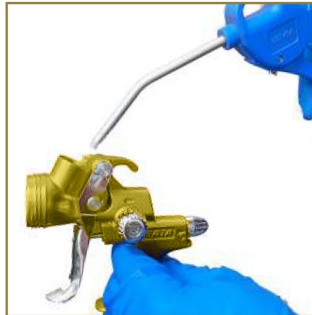
14 - Rinse the spray gun body and the paint channel with clean water. 15 - Dry using an air blower.
