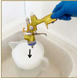
2 - Place the spray gun in the container.
