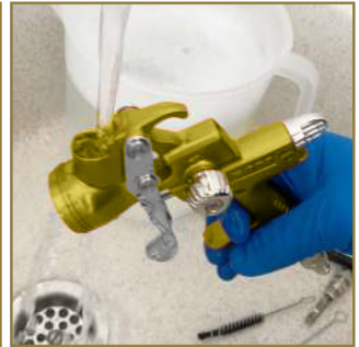
13 - Clean the spray gun body and the paint channel using the cleaning brushes. 14 - Rinse the spray gun body and the paint channel with clean water.
