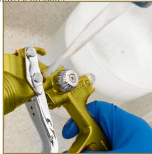
13 - Clean the spray gun body and the paint channel using the cleaning brushes. 14 - Rinse the spray gun body and the paint channel with clean water.
