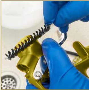
13 - Clean the spray gun body and the paint channel using the cleaning brushes. 14 - Rinse the spray gun body and the paint channel with clean water.
