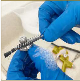
11 - Clean the nozzle on both sides using the cleaning brushes.
