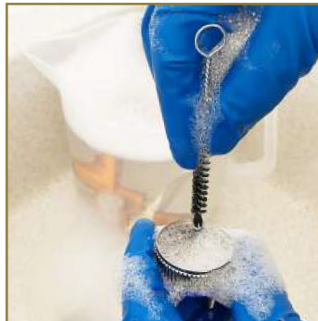
5 - Clean the air cap on both sides using the cleaning brushes.
