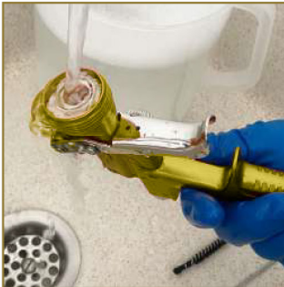
14 - Rinse the spray gun body and the paint channel with clean water. 15 - Dry using an air blower.
