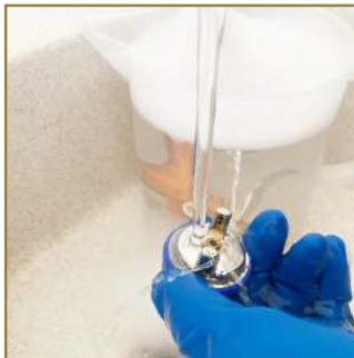
6 - Rinse the air cap on both sides with clean water.
