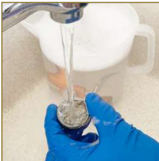
6 - Rinse the air cap on both sides with clean water.
